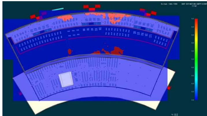
With a fire safety concept initially designed to extract smoke from the entire building via the large reading space, the choice was made for zone-specific cutting with a fire safety system specific to each zone. In the end, the architect concept and fire protection concept are diametrically opposed.
