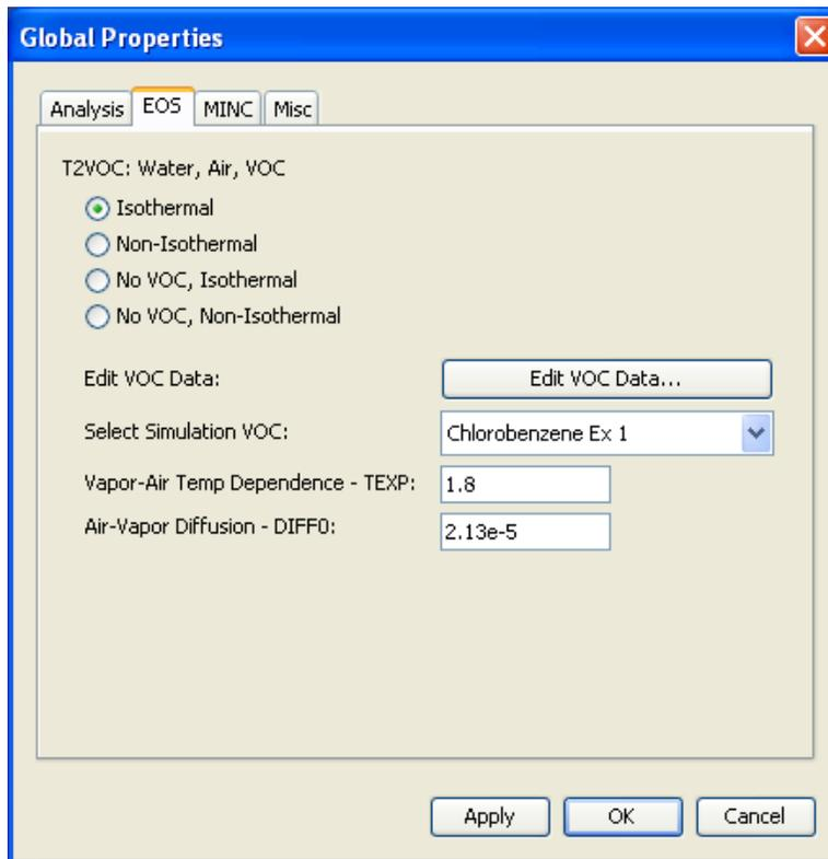
**Figure 3: T2VOC Simulation Parameters**
